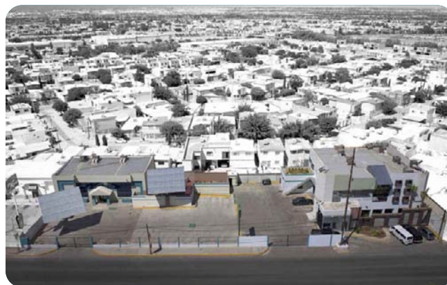
Heliostatic photovoltaic panels with installed capacity of 16 Kw, which will generate more than 43,000 Kwh per year.
